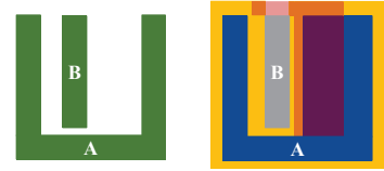
Figure 4: A side boundary of a feature not protected by a spacer results in a side overlay.
