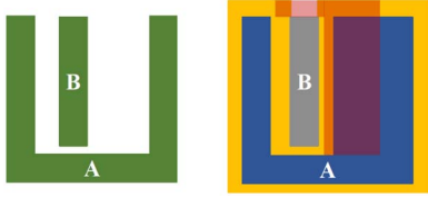
Fig. 4. Side boundary of a feature not protected by a spacer results in a side overlay.
